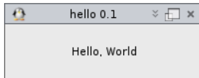
Code Snippet 1: A “Hello World” GTK+ GUI Application
